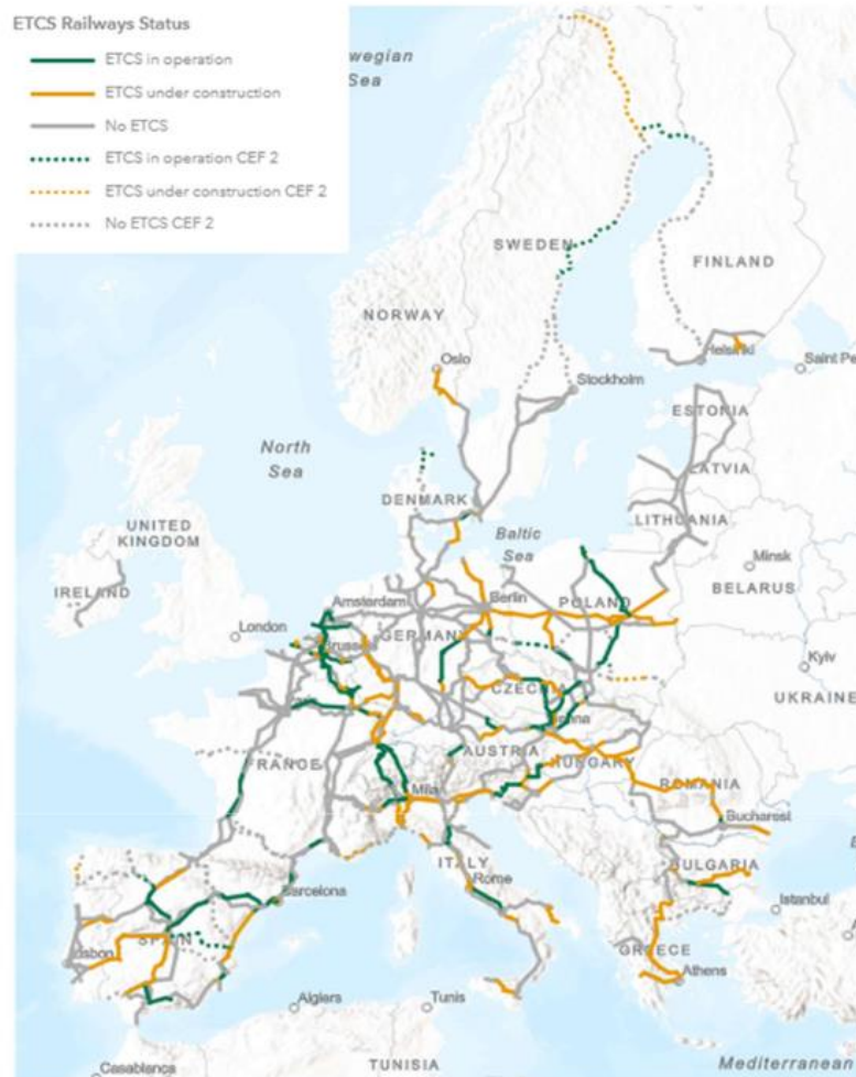
Figure 4 - ETCS deployment status in CNC – 06.2022 (source: ERTMS 2nd Work Plan of the European Coordinator)
